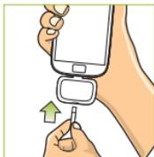
Tap the Gmate™ On app to enter. (If not installed, please see page 16.) Plug your meter to the USB jack of your mobile device. When the meter's power indicator is on, insert the test strip into the test strip port of the meter. Make sure the Gmate logo of the test strip is facing up.
